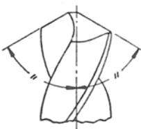
When this condition applies, the chisel edge of the drill is off center to the axis resulting in oversized holes and submitting both drill and machine to undue strain.
